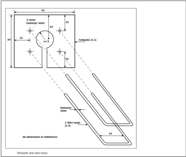
FIG. 8 STEEL TEMPLATE AND WIRE LOOP
