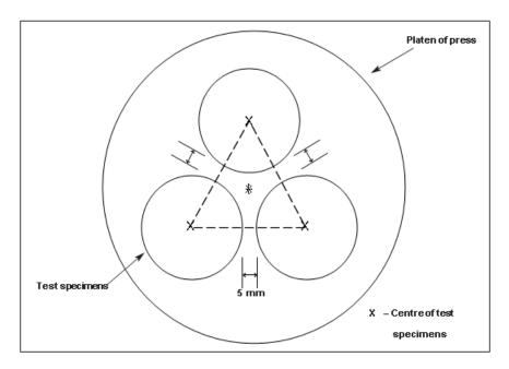
FIG.4 PLAN VIEW OF TEST SPECIMENS AND PLATEN
