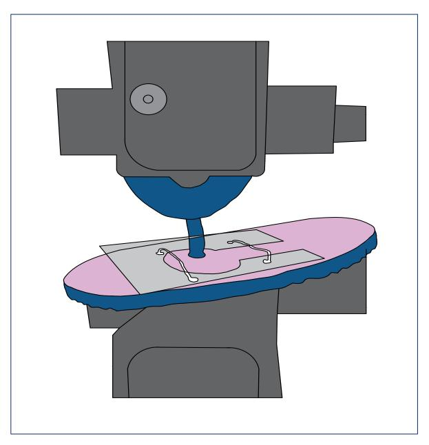
Fig. 9 Illustration Diagram For Clamping of Toe Post Strap in the Tensile Machine
