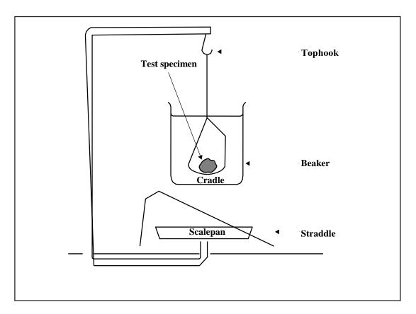
FIG. 3 A CRADLE SUSPENDED FROM A TOP HOOK
