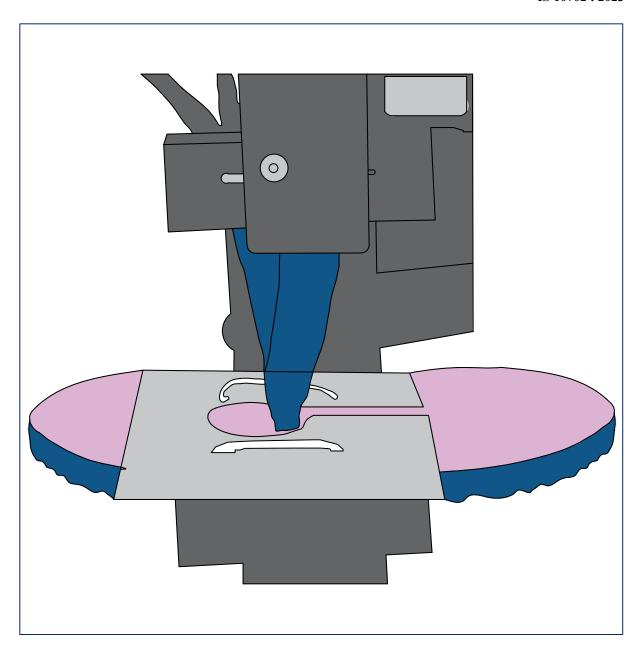
$Fig.\ 10\ Illustration\ Diagram\ For\ Clamping\ of\ Rear\ Strap\ in\ the\ Tensile\ Machine$
