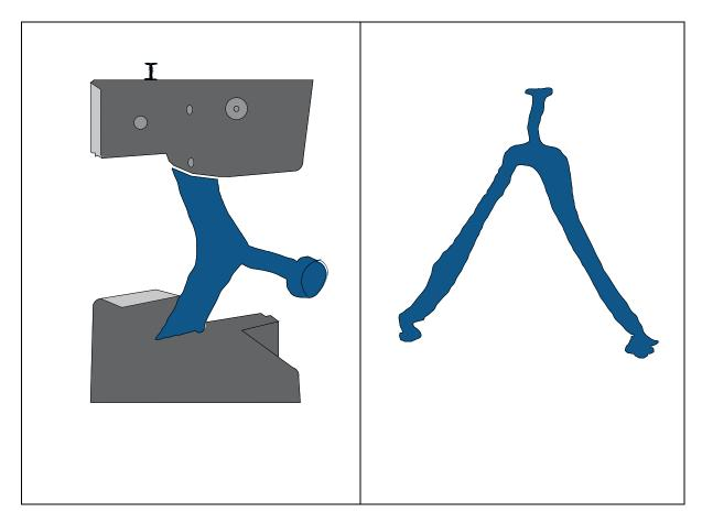
Fig. 6 Illustration Diagram For Clamping of Strap to Toe Post Sample to be Fixed in Tensile Testing Machine
