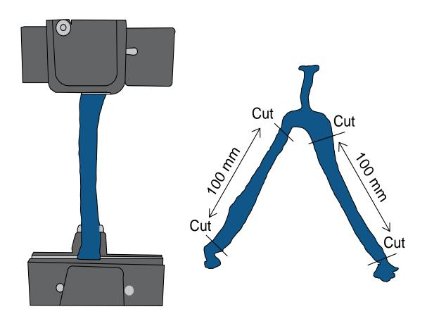
Fig. 7 Illustration Diagram For Clamping of Strap-to-Strap Sample to be Fixed in Tensile Testing Machine
