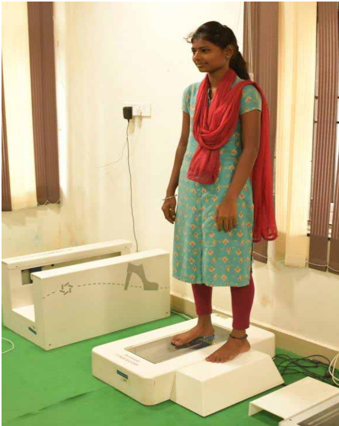
Scanning of Bottom Profile of Foot using “Flat Foot Scanner”
