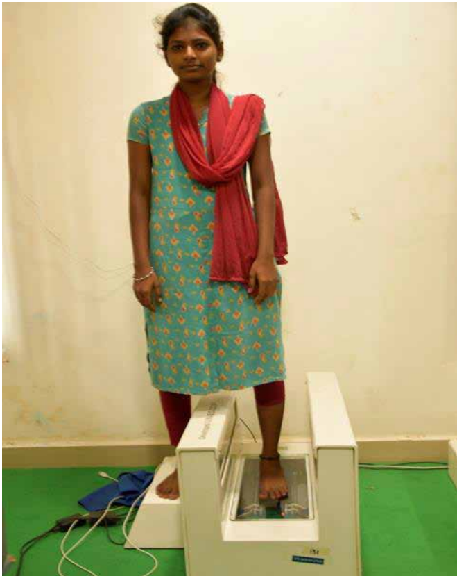
3D Scanning of Foot using “Ankle Scanner”
