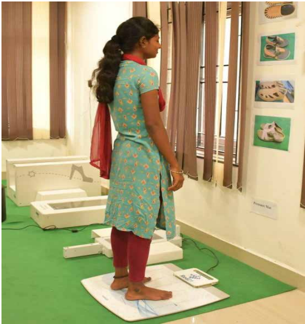
“PODOPRINT PRESSURE MAT” to measure Plantar Pressure of the patient
